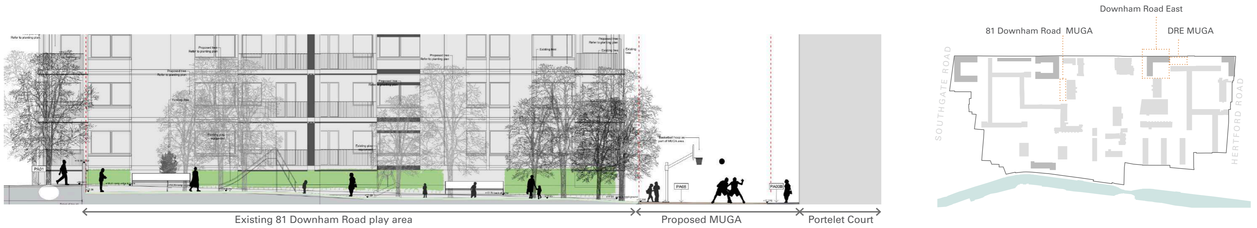
Above: section showing proposed 81 Downham Road Mixed Use Games Area in context with the existing play area and the proposed 81 Downham Road building behind
