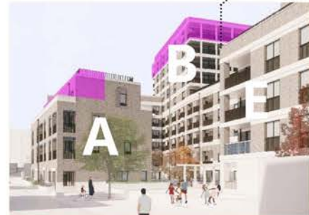
Proposed scheme - Blocks A & B (Purple shade shows additional mass proposed while the dotted line indicates the former 5th floor to Block E, removed in the amended scheme)
