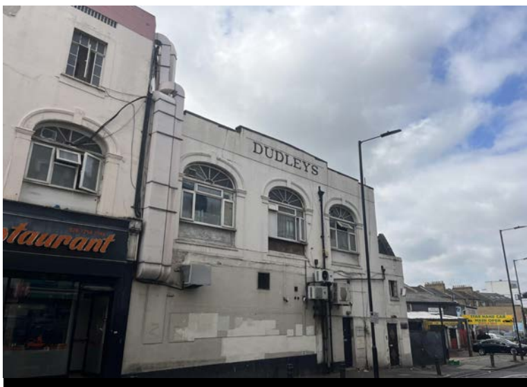
✗ Figure 3.3 – Unacceptable highly visible ducting on the public frontage of a building.
