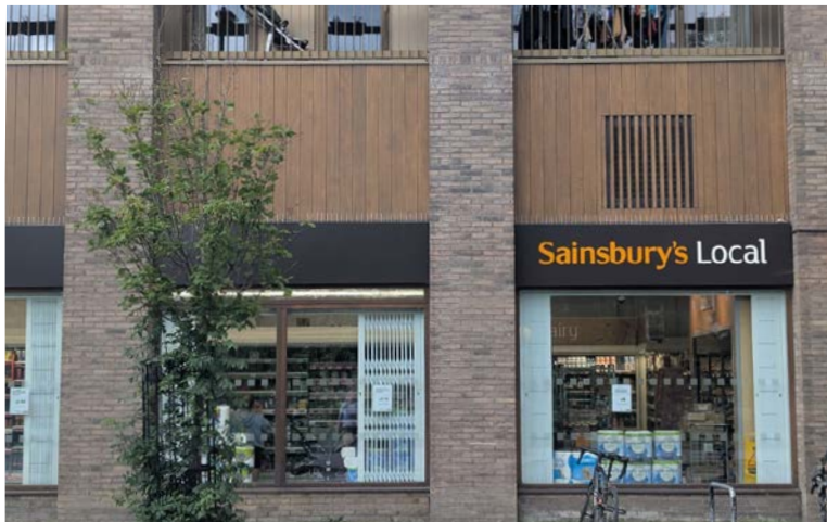
✓ Figure 5.11 – A contemporary shop front featuring translucent external shutters, minimal use of decals and some traditional shop features including a fascia which does not interrupt the architecture of the building.
