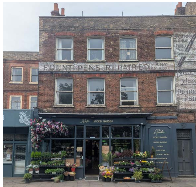
✓ Figure 7.6 – Ghost signs were originally painted with oil-based house paints. The paint that has survived the test of time most likely contains lead, which keeps it strongly adhered to the masonry surface.
