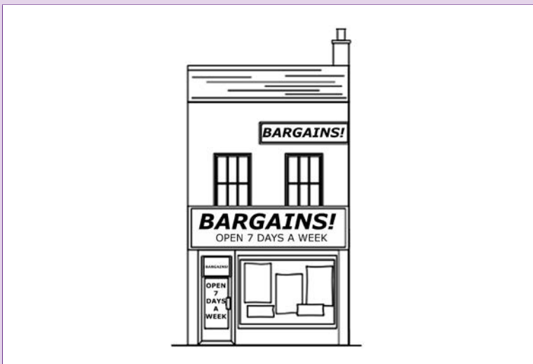
✗ Figure 5.2 – Fascia hidden by large scale lettering and cluttered signage that is not in keeping with the shopfront design.
