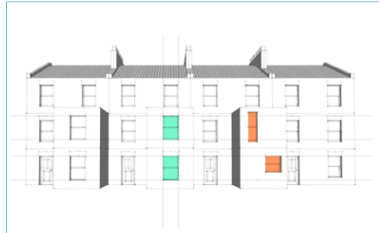
Figure. 3.14 – Illustration demonstrating windows on an extension which aligns with the openings on the existing building (green) and windows that are off centre which results in an insensitive alteration (red).
