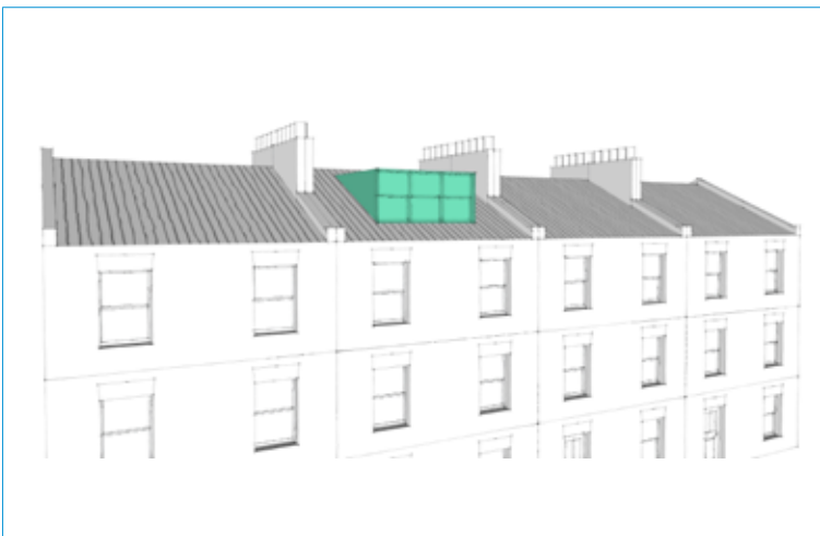
Figure 6.9 – Single dormer window aligned symmetrically within the plane of the roof. Width of dormer not to exceed half the width of the roof.
