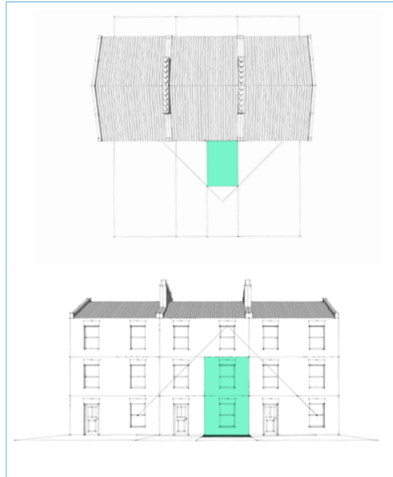
Figure 3.7 – Example of an extension demonstrating the impact of the 45 degree rule.
