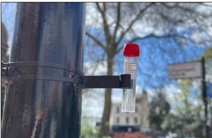
Figure 11: \text{NO}_2 diffusion tube attached to a sign post in Lower Clapton
