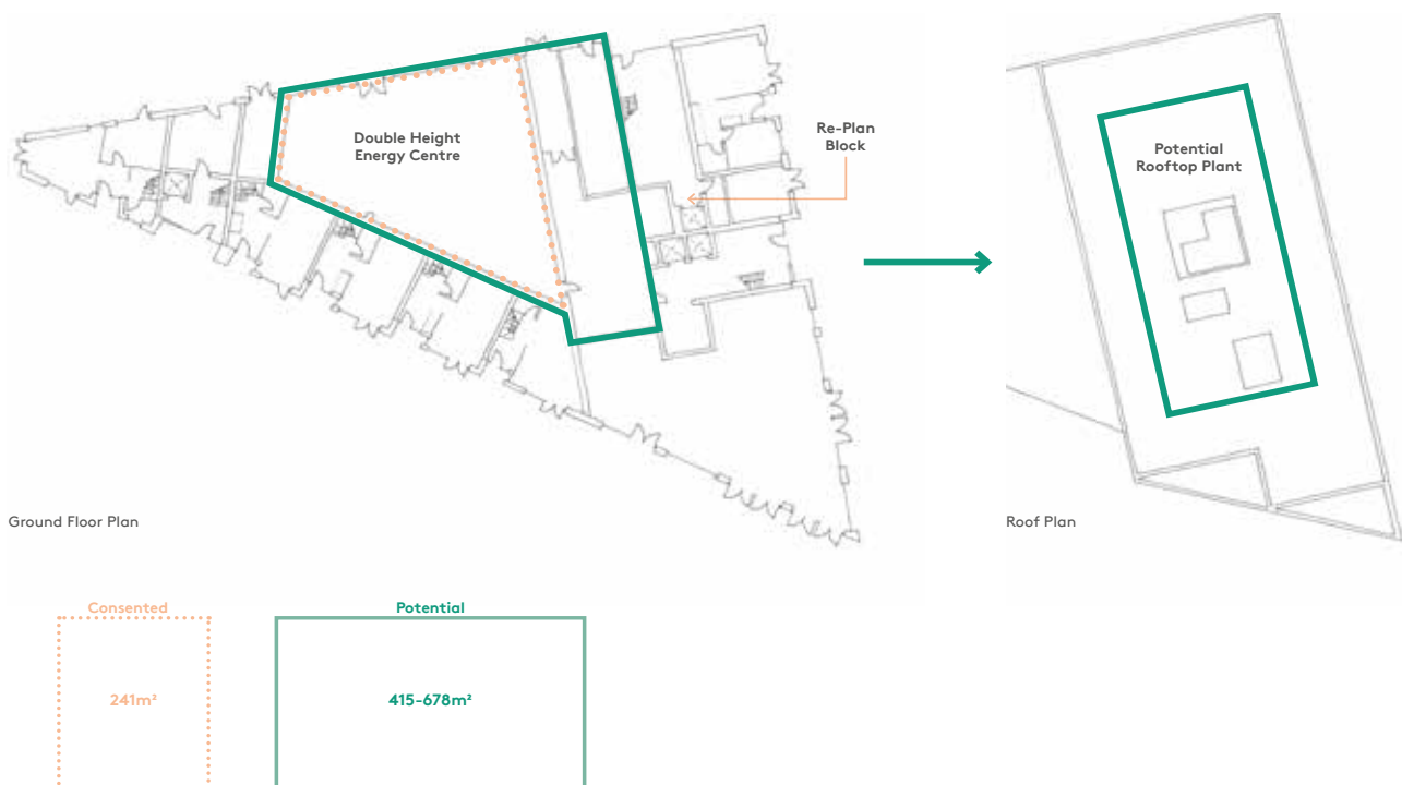
Diagram showing potential increase of energy centre compared to original scheme, including requirement for roof plant to achieve a low carbon solution.
