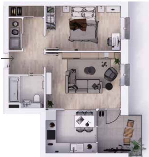
Open plan example for 1 bedroom flat with sliding partition to kitchen area for built-in flexibility.
