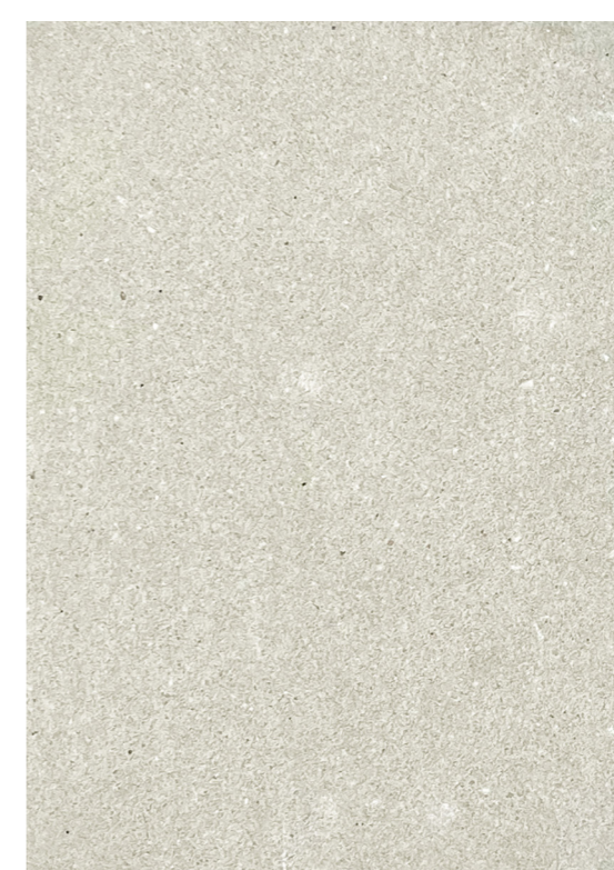
Fair faced in-situ concrete
