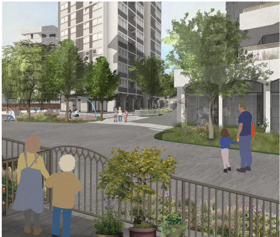
We have removed the low wall that was proposed in-front of the ground floor Halstead Court homes. In response to feedback we propose a new railing, gate and planter to each home.
