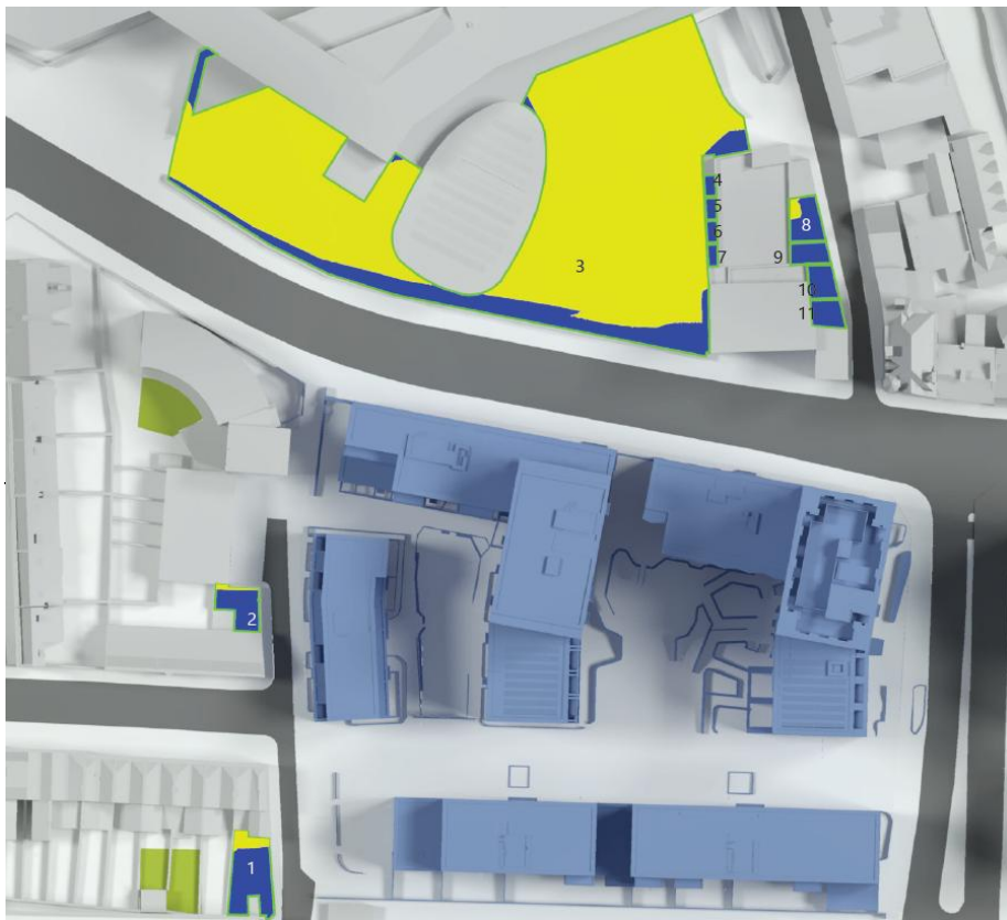
Image 8 - BRE 2-Hour sun contour analysis to the neighbouring amenity spaces in the proposed condition
