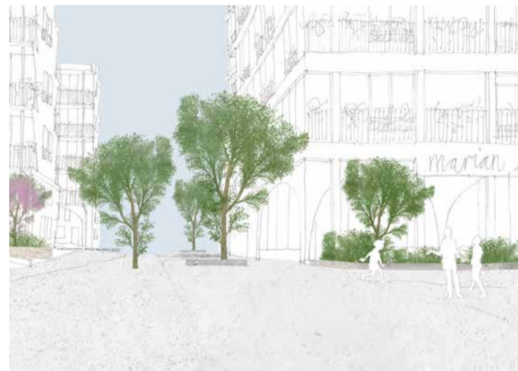
A new East West walking and cycling route. No through traffic, tree acting as bollard and the only parking for disabled residents and access for delivery, refuse and fire trucks.
