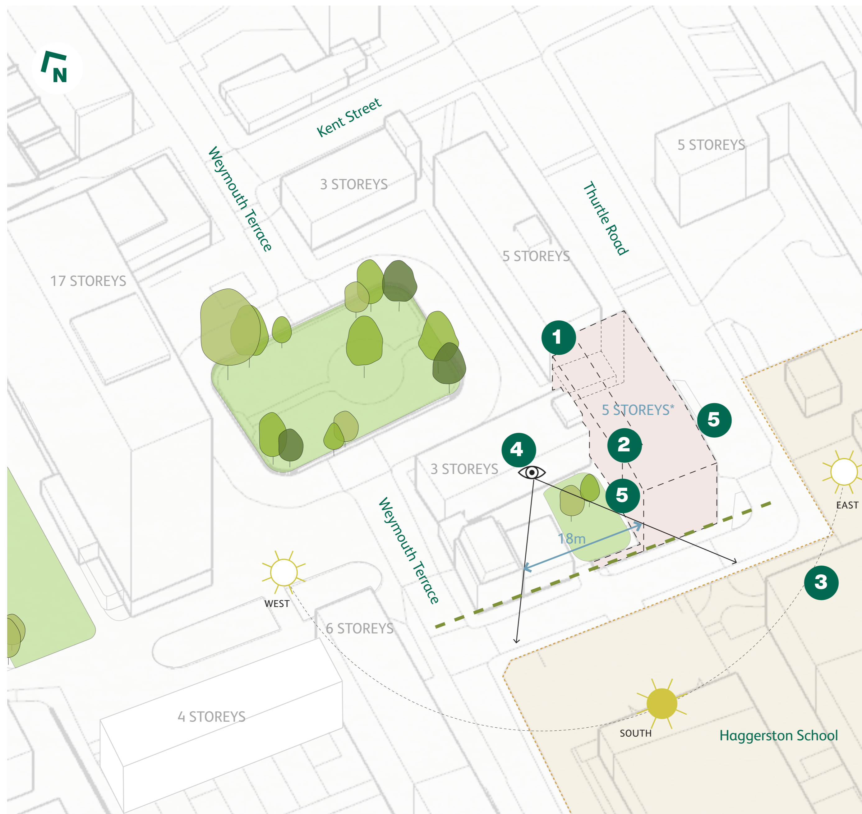
Axonometric of the site, showing in pink the initial proposed building massing * New 5-storey construction will be taller than existing 5-storey buildings to meet current design guidance and building regulations.
