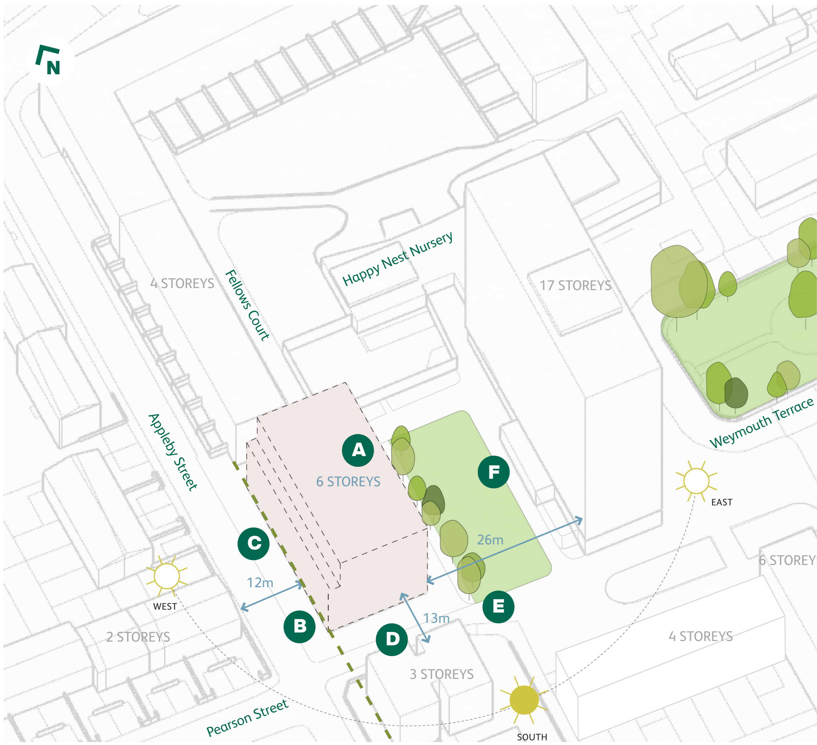
Axonometric of the site, showing in pink the initial proposed building massing
