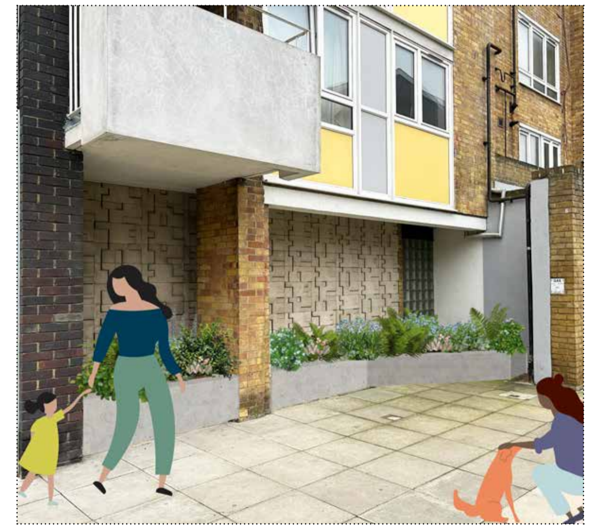
View 1: illustration of potential tower planter. The existing wall contains a vertical gas pipe that cannot be moved
