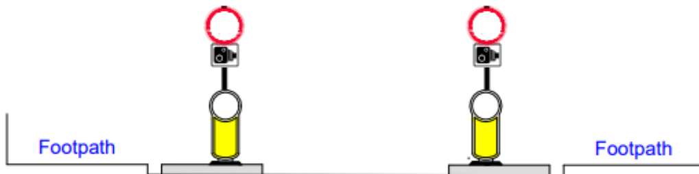
View showing "no motor vehicle" signing and plain face reflective bollards located on traffic islands, as you approach.
