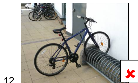
Poor support and poor security
