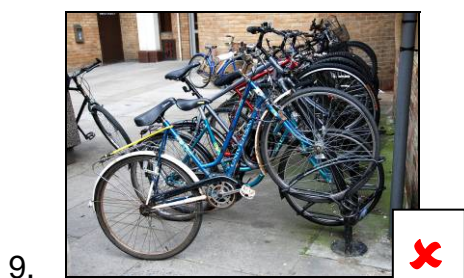
Requires the bicycle to be lifted + poor security
