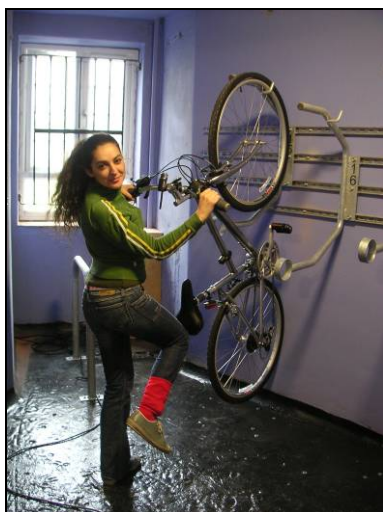
Retro-fit solution - hanging racks used in a confined space – note the Sheffield rack under the window provided for those unable to lift their bicycle
