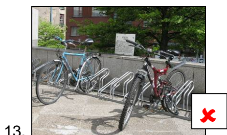
Poor support and poor security
