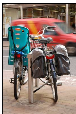
At least 1000mm is needed to accommodate bicycles with child seats and panniers ...
