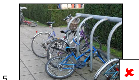
Poor support and poor security
