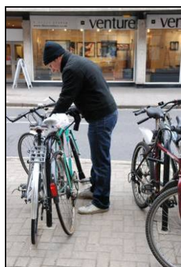
Stands 1000mm apart allow cyclists room to lock their frames in comfort
