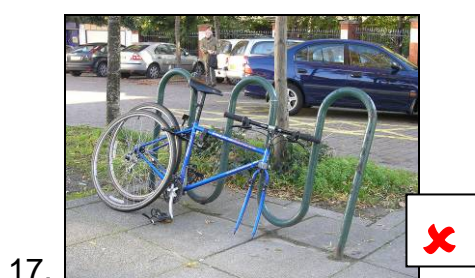
Poor support and security when used as intended (i.e. bicycle slotted in at right angles to stand)
