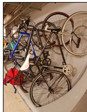
Channelled racks with hoops to lock wheels and frame
