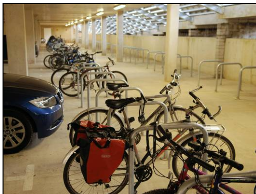
Good quality parking within a secure area - note the incursion of the car into cycle parking space: this should be designed out from the beginning
